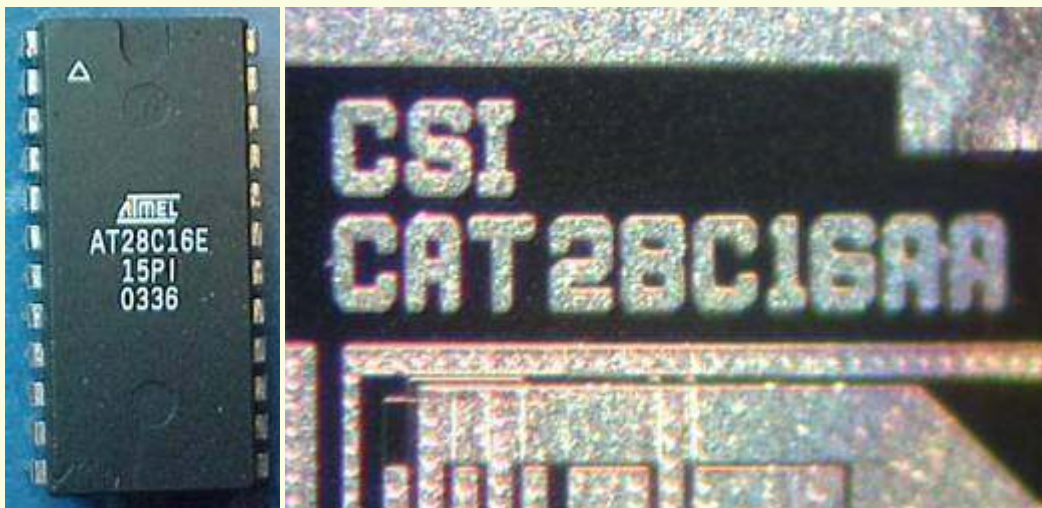
Counterfeit - Marked Atmel with Catalyst Die
